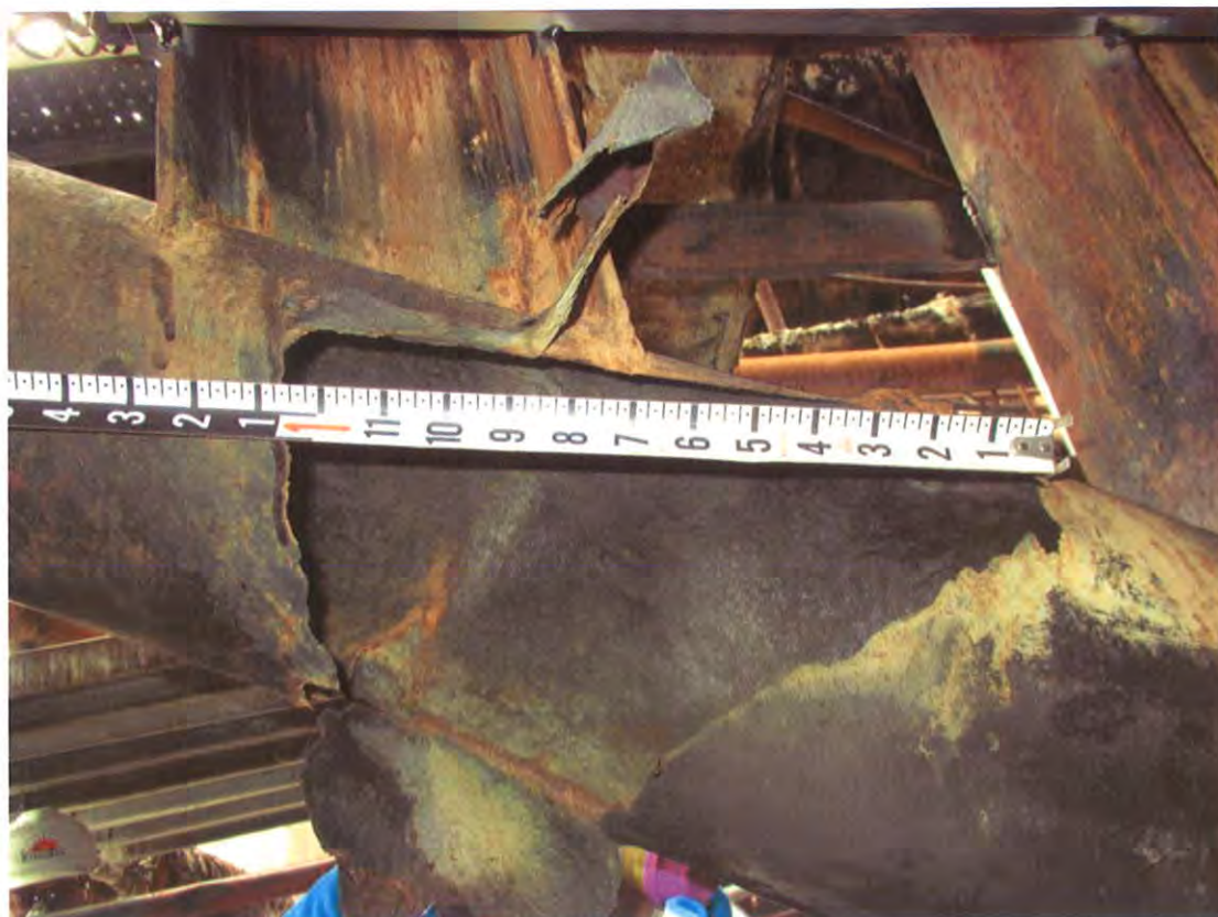
Figure 8. Close-up photograph of the ruptured pipe component taken during the inspection prior to removal.
