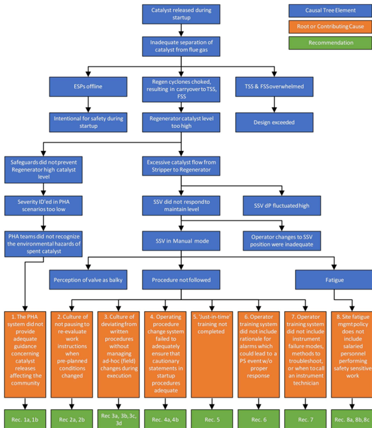
Figure 2: Causal tree of November 24-25, 2022, Catalyst Release Incident
