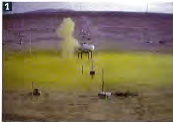
(1) Jack Rabbit I: Rapid phase transition behavior. [Photos by U.S. Department of Homeland Security (DHS)—Chemical Security Analysis Center (CSAC).]
