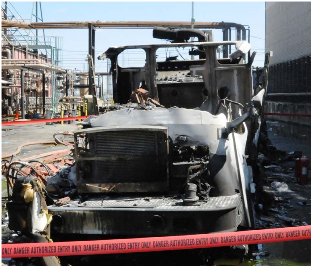
Figure 1. The burned remains of the fire truck that was consumed by the fire. A firefighter was in the cab when the vapor cloud ignited. The fire truck was positioned approximately 65 feet from the leak location.
