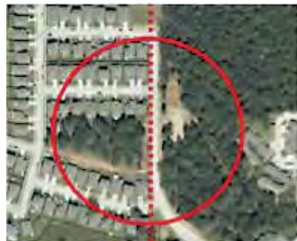
Example of a Potential Impact Radius of a pipeline incident shown on an aerial map (assumes the pipeline rupture occurs at the center of the circle)
