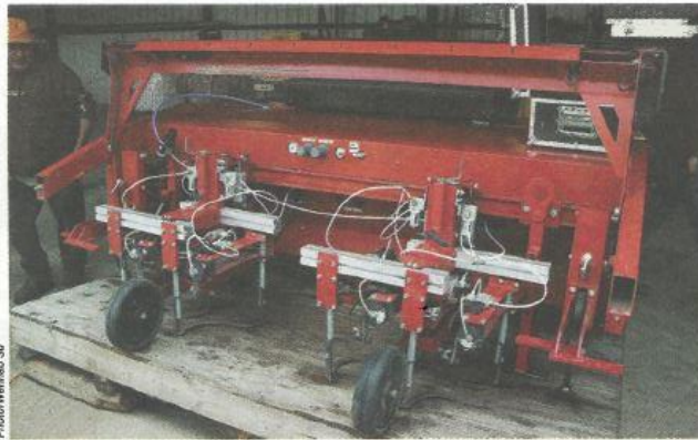
This Steketee automatic weeder was on display at recent field day. Equipment like this is designed to remove weeds from row crops without damaging the crop.
