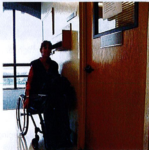
Figure 15: Chart box affixed to an examination entrance door, shown as eye level to a wheelchair or scooter user.
